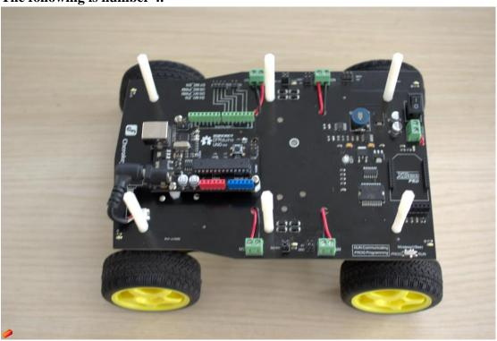
5. Install the expansion plate board
