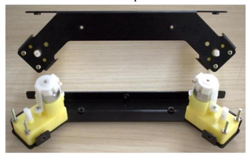
2. To fix the connecting rod on the edge of the side-panel and install wheels *Friendship reminded:* It might be better to welding polarity lines on the motor before to fix the connecting rod. Lines set aside a certain length to connect the microcontroller.
